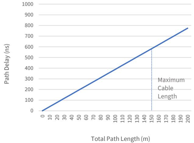
\* **Test conditions:** Propagation time and signal attenuation measured on 50 m of Belden H155 and 150 m of H2010 Ultraflex coaxial cable. Graph calculated based on the known assumptions that (a) if cable specifications and frequency are constant, path attenuation has a linear relationship to path length and (b) if cable specifications are constant, path delay has a linear relationship to path length.
