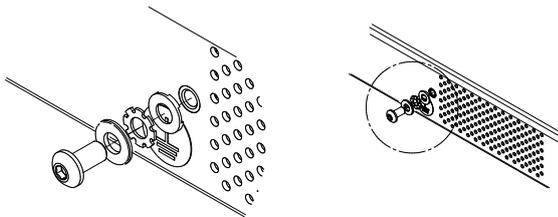
This connector must be wired to an equipotential bonding bar (earthing bar). Connection is possible on the left hand side (frontview) of the housing. The mounting parts (without cable) are included in the scope of delivery.
