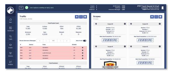
PTP Track Hound is Meinberg's powerful PTP monitoring toolkit that provides a wealth of functions for monitoring PTP clock networks. These functions support both native PTP functions for measuring path delay and asymmetry and acquiring diagnostic data as well as a variety of proprietary extensions integrated in compliance with the IEEE 1588 standard.
