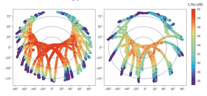
Sample skyplots of carrier-to-noise ratios in dB for reception of GPS (*left*) and Galileo (*right*) taken using Meinberg GNS-UC receiver under ideal conditions (no signal obstacles within 10 meters) at angles of up to approx. 85° in all directions from zenith to horizon.
