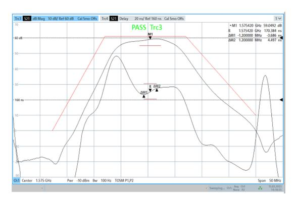
Frequency-response curve illustrating the production benchmark (**red**), the gain curve with the center frequency of 1575.42 MHz (**M1**), and the delay curve (**R**) with delay variations between 1574.22 MHz (**ΔM1**) and 1576.62 MHz (**ΔM2**)
