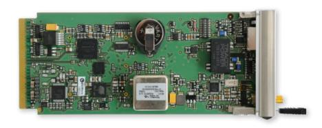
Meinbergs built-in MRS system can handle a wide range of reference sources like GPS, Time of Day, 1PPS, 10 MHz in a configurable, user-prioritized way. This improves flexibility and reliability, allowing you to set up a primary reference source and back up references.
