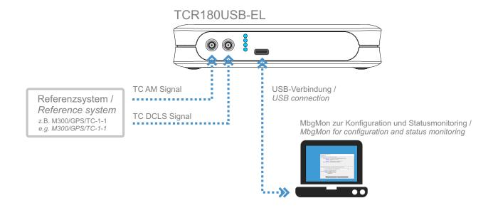
Figure: Synchronization of the TCR180USB-EL via an M300/GPS/TC-1-1 as reference system
