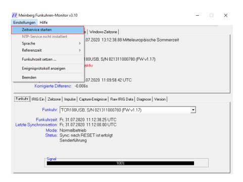
After all necessary IRIG settings have been made, the time service can be started.
