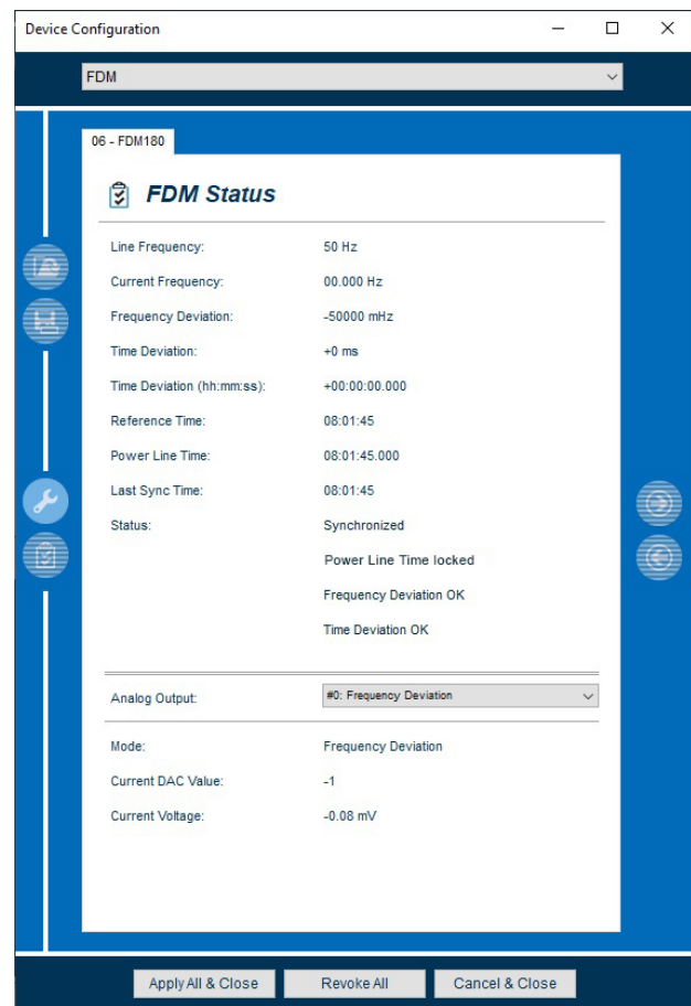
Figure 87: FDM – Status Monitoring
